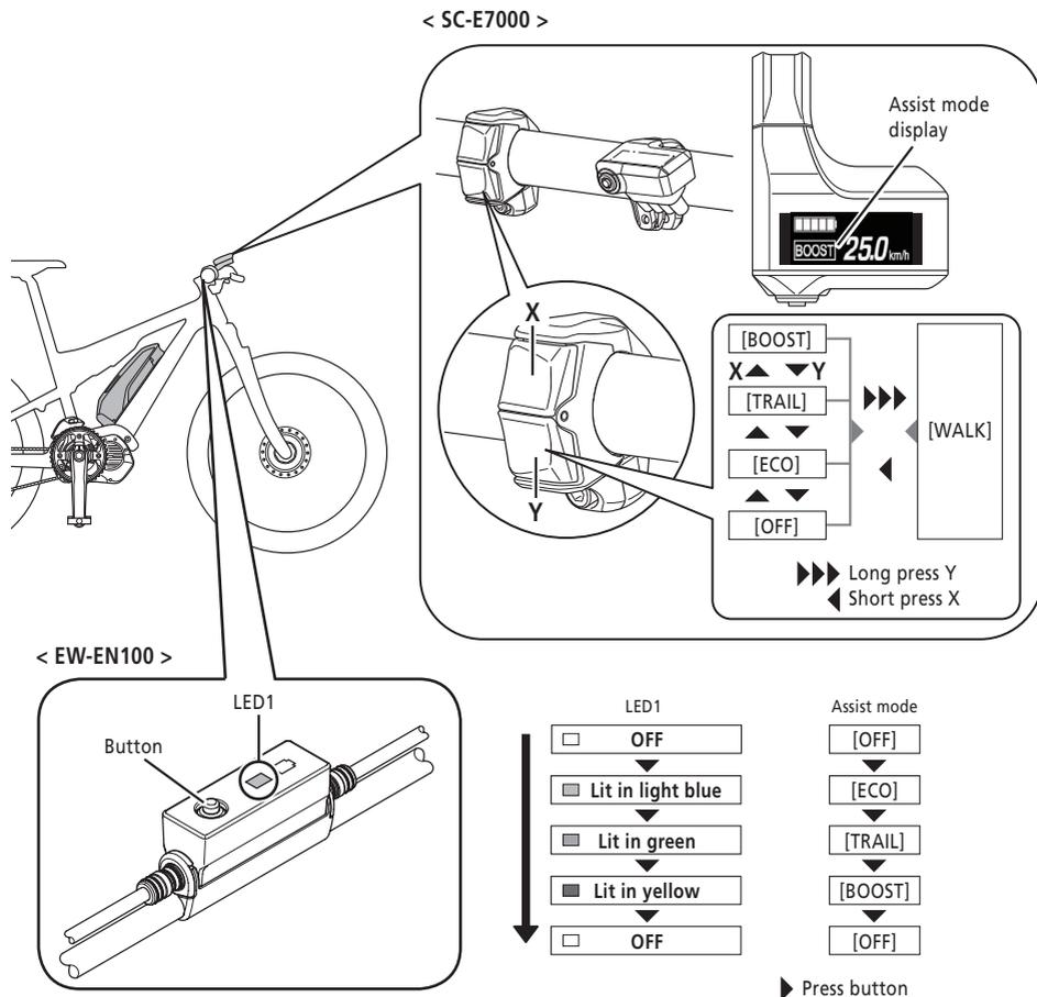
\* To change to the [WALK] assist mode, it is necessary to operate the above assist switch.
