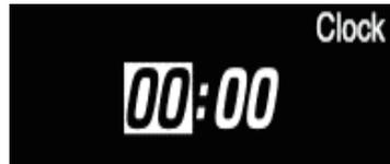
3. Pressing the function button enables the set value and moves you to the minutes setting.
